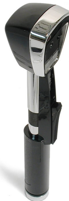
Figure 3: Copeland retinoscope. Putting the sleeve up provides the plane mirror effect.
